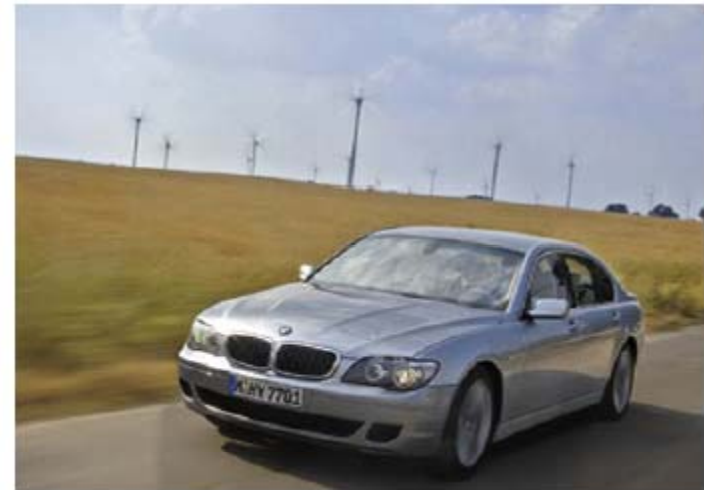
Figure 20.26. BMW Hydrogen 7. Energy consumption: 254 kWh per 100 km. Photo from BMW.
