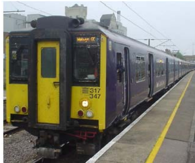
Figure 20.4. This 8-carriage train, at its maximum speed of 100 mph (161 km/h), consumes 1.6 kWh per 100 passenger-km, if full.
