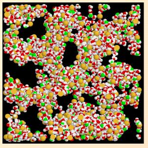
Percolation theory relates the effective diffusivity to the fraction of bonds that are blocked to diffusion.
