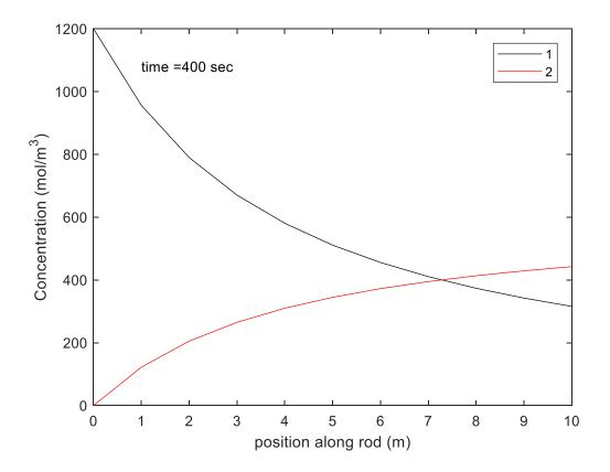
The concentration of A at the pipe outlet at steady state is >> Tmat(12,4001,1) ans = 315.5597
