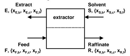
You are given all four flow rates and the compositions of the Feed (F) and Solvent (S) streams. Your task is to determine the composition of the two exiting streams, the Raffinate (R) and Extract (E).
