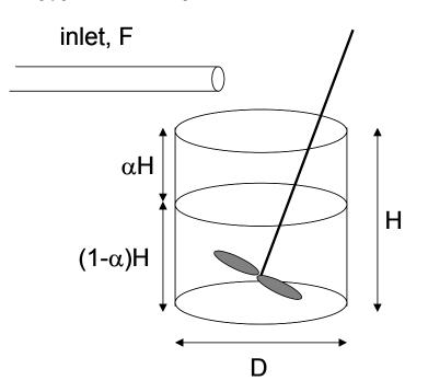
The tank is cylindrical with height, H, and diameter, D. The two-cell model assumes that the concentration is homogeneous in each cell, but different between cells.  $\alpha$  is the volume fraction of the top cell. The inlet volumetric flow rate is F, with concentration C<sub>in</sub>.
