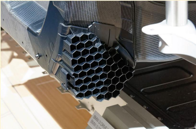
Honeycomb structure made of injection-molded plastic fixed onto a carbon-fiber-reinforced polymer chassis on a BMW i3.
