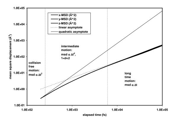
In this log-log plot, we can more clearly observe the exponent relating the elapsed time to the MSD. At short times, the curves follows a quadratic (m=2) limit. At long times, the curves follow a linear (m=1) limit.
