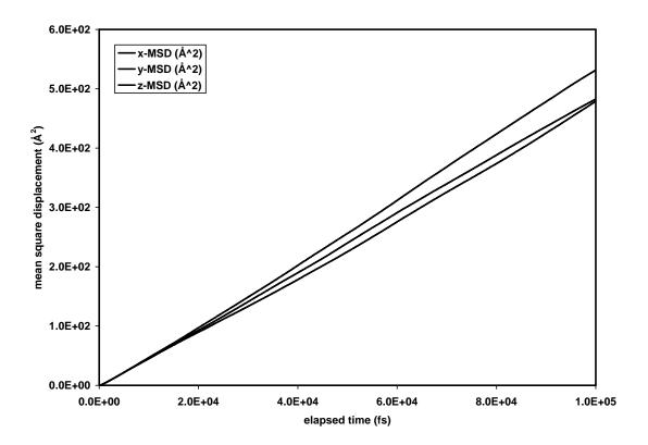
In this plot, you observe nonlinear behavior at short time and linear behavior at long times. The variation between x, y and z in an isotropic material is an indication of the uncertainty in the measurement. The slope of the long-time linear part of these curves is 2D. The dimensionality here is considered as one since we analyze the three dimensions independently.
