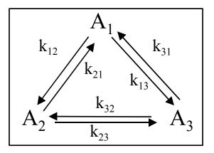
In this picture, the A's are concentrations of the three species and the k's are rate constants. An example of this system is the kinetic equilibrium between para-, meta-, and ortho-xylene.
