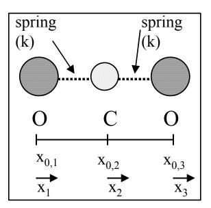
We model the interaction between molecules as Hookian springs. For a Hookian spring, the potential energy,  ${\sf U},$  is
