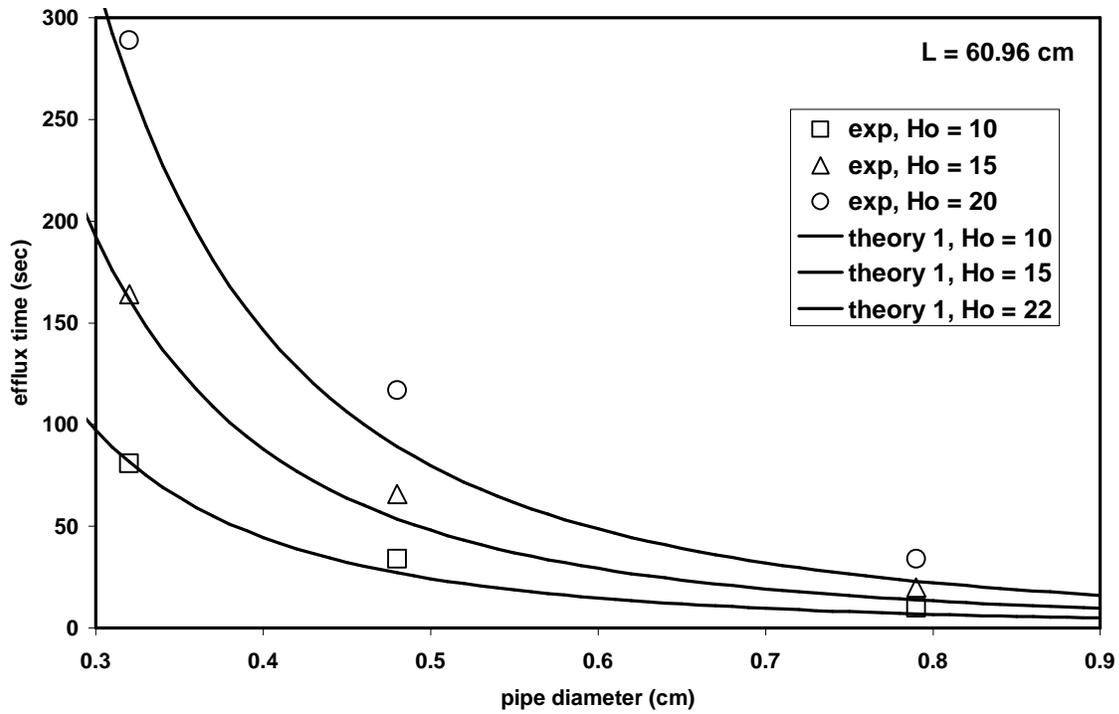
Figure Three. Efflux time as a function of pipe diameter, using the pipe of Length 60.96 cm and initial water heights of 10, 15, and 20 cm. The theory lines represent Case One, equation (8).
