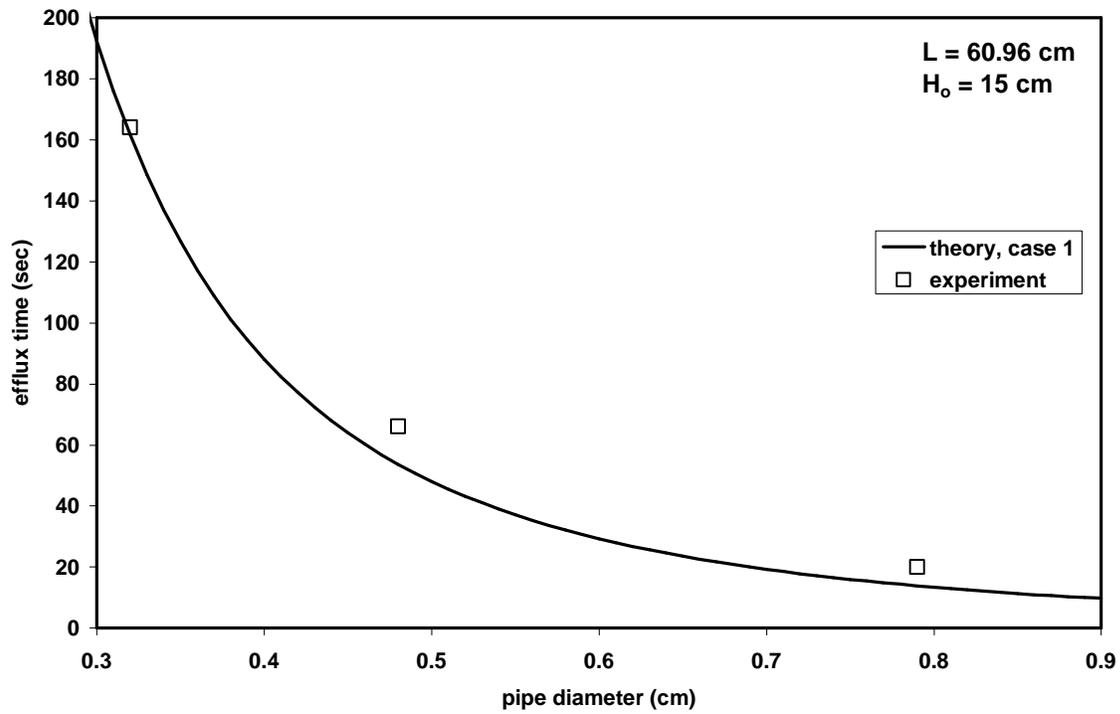
Figure One. Efflux time as a function of pipe diameter, using the pipe of Length 60.96 cm and an initial water height of 15 cm. The theory line represent Case One, equation (8).
