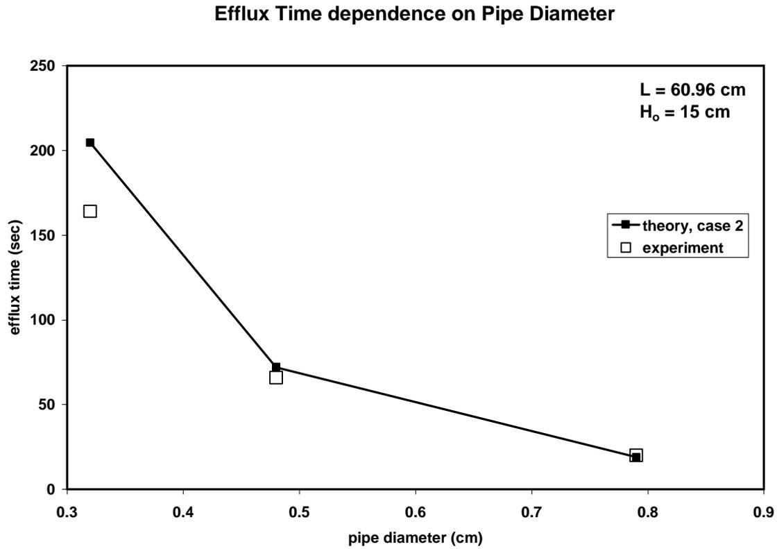
Figure Two. Efflux time as a function of pipe diameter, using the pipe of Length 60.96 cm and an initial water height of 15 cm. The theory line represent Case Two, equation (16).
