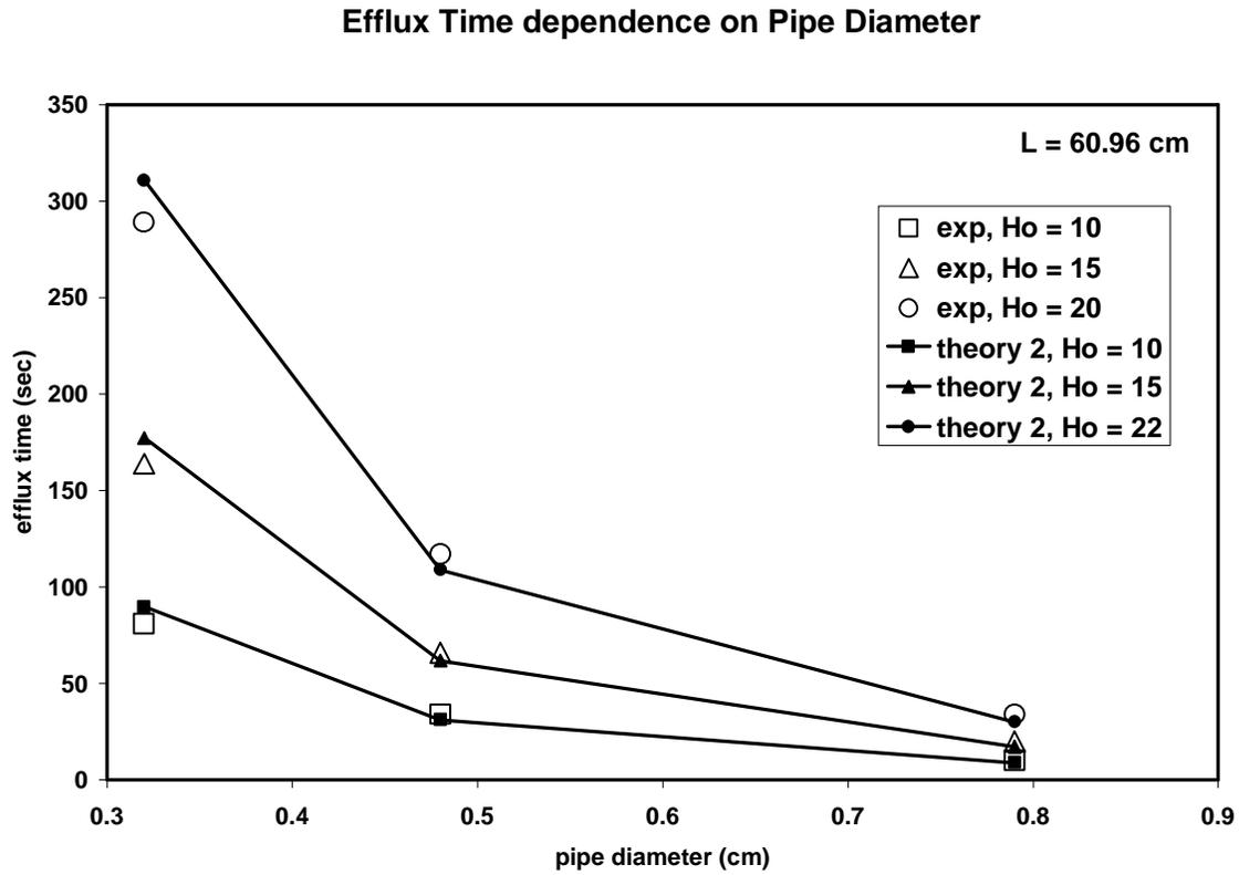
Figure Four. Efflux time as a function of pipe diameter, using the pipe of Length 60.96 cm and initial water heights of 10, 15, and 20 cm. The theory lines represent Case Two, equation (16).
