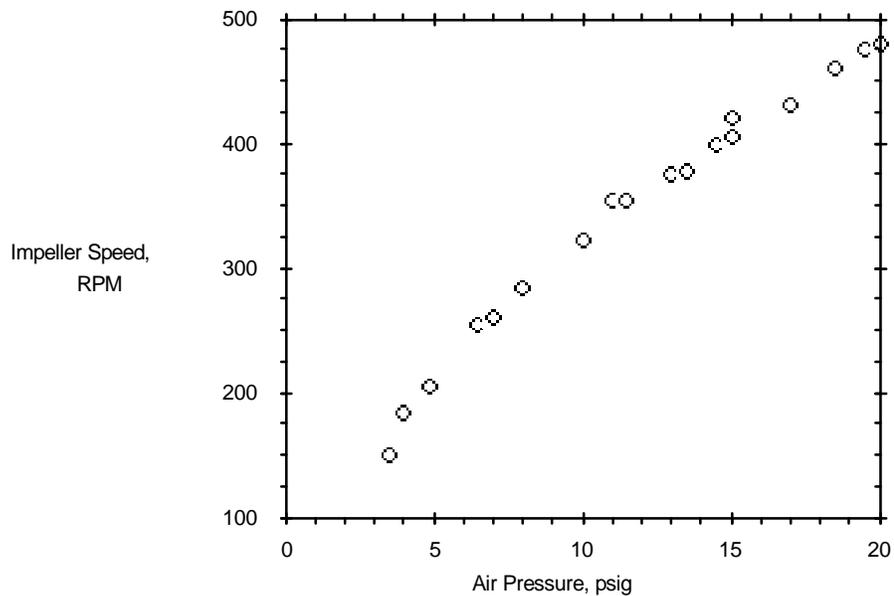
Figure 1. Air Impeller Performance Characteristics
