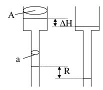
where a and A are cross-sectional areas. Express  $\Delta H$  in terms of R, a, A. (The underlying principle here is conservation of volume. The volumes in both tubes are equal.)
