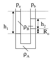
$R_o$  is the initial difference between fluid levels at zero pressure difference. If the pressure at point a is the same as the pressure at point b but the amount of B-fluid in the two legs of the manometer is different (so  $h_1 \neq h_2$ ), find  $R_o$  in terms of  $h_1, h_2, \rho_A, \rho_B$ .
